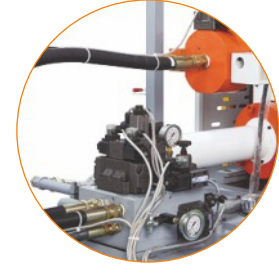
Double proportional control oil circuit, pressure and speed can be adjusted automatically
